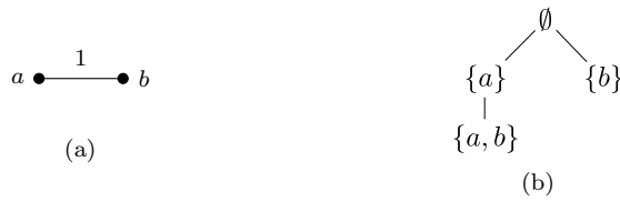
Fig. 6: (a) A graph and (b) its corresponding enumeration tree obtained with Algorithm A_1 .
