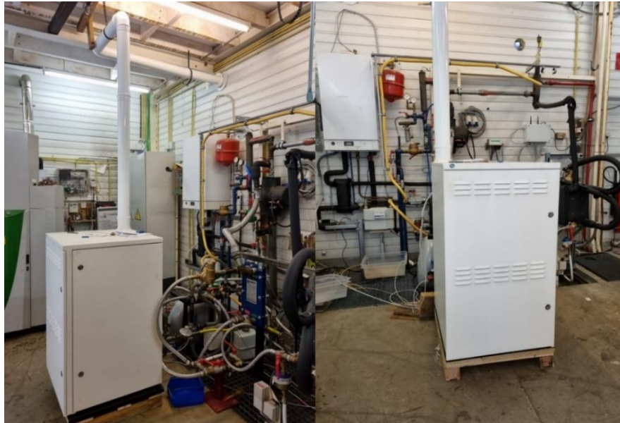
Figure 1. Tested mCHP SOFC in ULiege laboratory facilities
