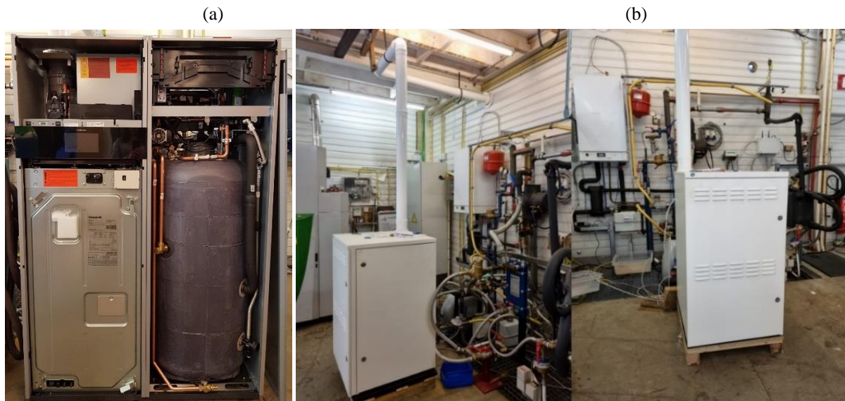
Figure 3. Tested fuel cell mCHP systems in the laboratory facilities. (a) PEMFC; (b) SOFC.
