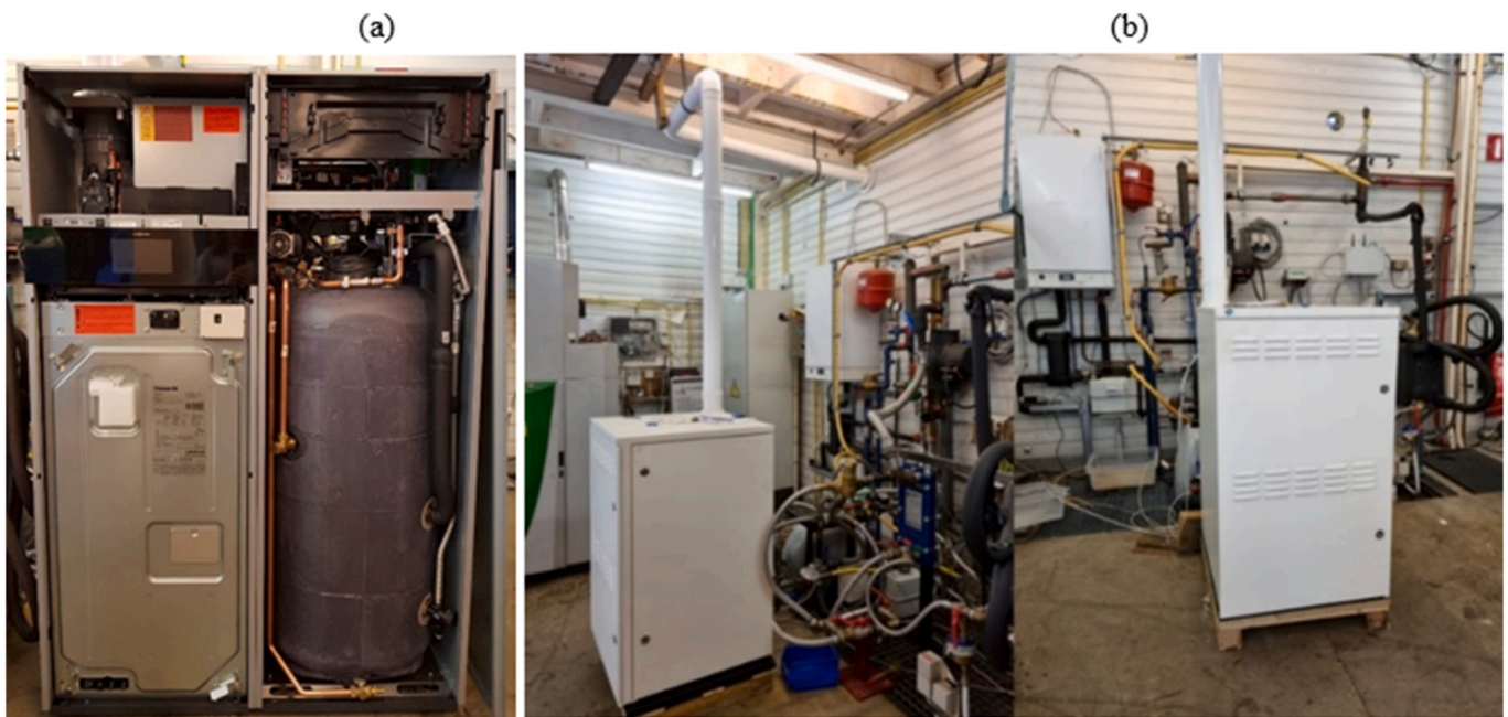
Fig. 3. Tested fuel cell mCHP systems in the laboratory facilities. (a) PEMFC; (b) SOFC.
