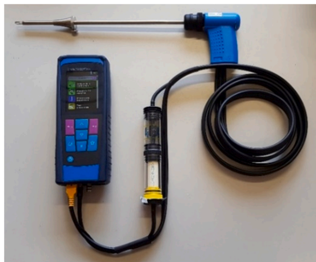
Fig. 4. 'Multilyzer STx' combustion analyser portable meter.
