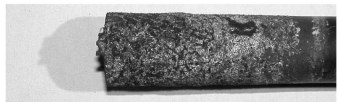
Fig. 6. Heat checking (borided steel, R5.5 s cycles).
