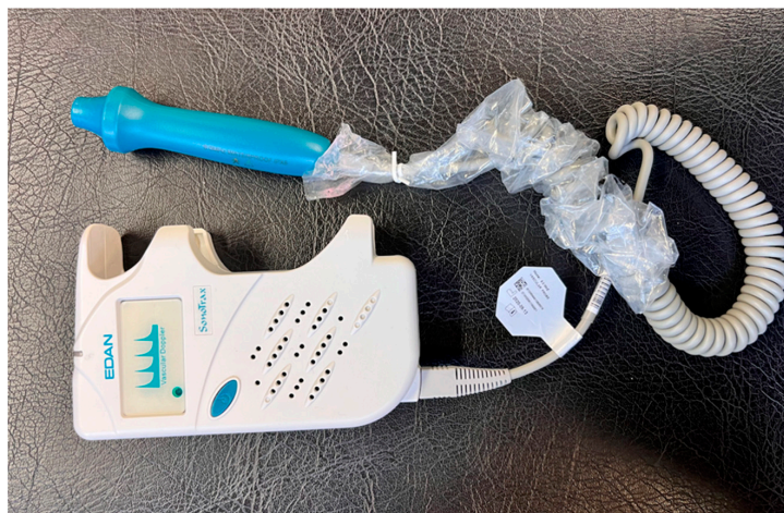
Figure 3. Audible Doppler device used to determine LOP.
