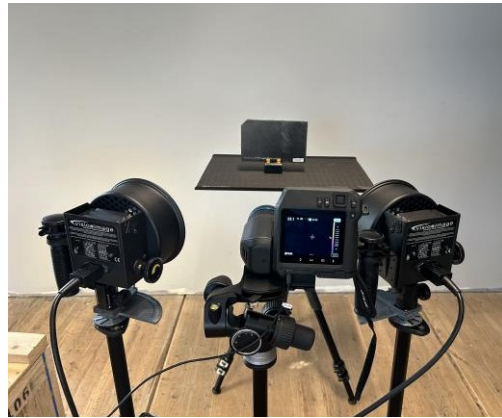
Figure 3. Experimental set-up with two halogen lamps, one CFRP benchmark and one thermal camera.
