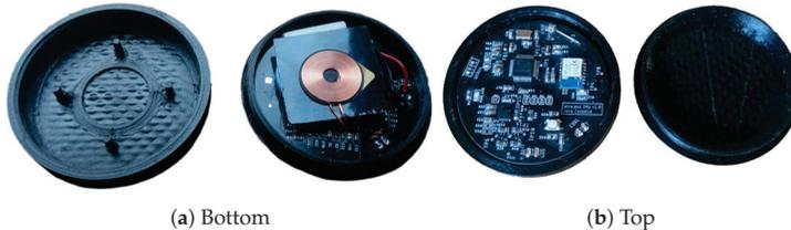
**Figure 9.** Result: sensor node in the 3D printed case. (a) Bottom side: wireless charging coil and battery. (b) Topside: IMU, microcontroller, and BLE chip.
